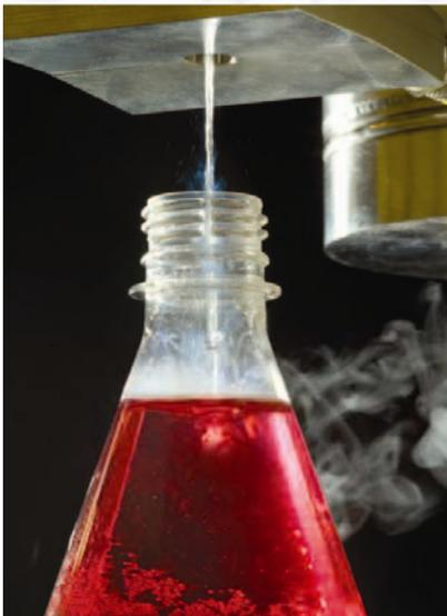
Vacuum Barrier's NITRODOSE® liquid nitrogen injection systems provide the most precise liquid nitrogen dosing to add strength to non-carbonated beverages for light-weight packaging and displace oxygen to extend shelf life.
