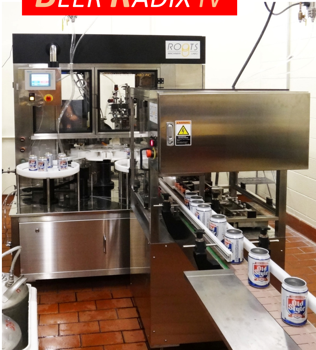
"Beer Radix IV" at MillerCoors pilot plant in Milwaukee, WI, USA. "Three head water rinser" is integrated in front of the Beer Radix.
