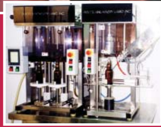
ガス飲料びん詰め機「ROOTS BF-III R」 / Gas beverage filler capper, by ROOTS
