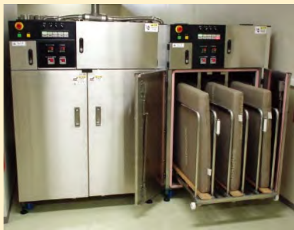
Used injector needle cutter and sanitizer, developed as derivatives of Self-Heating can.
